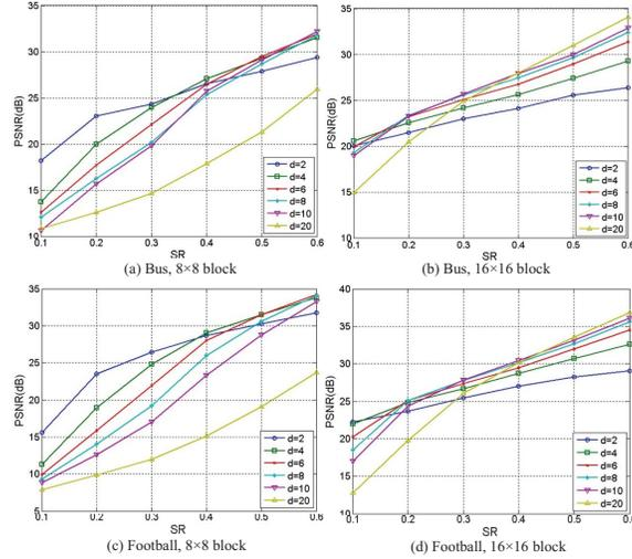
Figure 7: The performance of the proposed scheme with different dimension  $d$ . (a): *Bus*,  $8 \times 8$ ; (b): *Bus*,  $16 \times 16$ ; (c): *Football*,  $8 \times 8$ ; (d): *Football*,  $16 \times 16$ .
